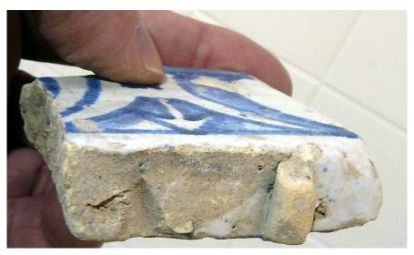
**Figure 16.** A fragment of tile that was never applied and still has adhered one of the supporting cylinders for firing upright (image: *Museu do Palácio da Bacalhôa* c. Associação de Coleções | The Berardo Collection).
